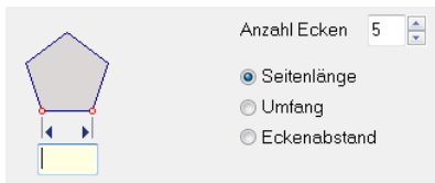
Measuring method 1: Measure the length of a side
